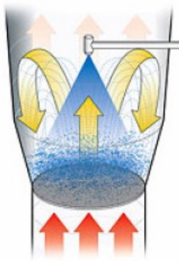
Principle: Batch fluid bed coating Top Spray
