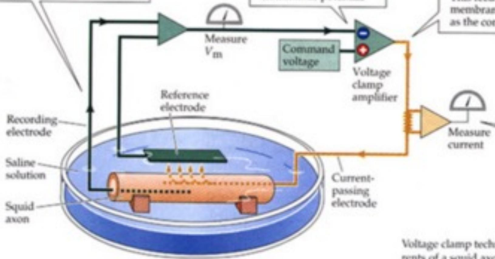
Voltage clamp technique for studying membrane currents of a squid axon.
