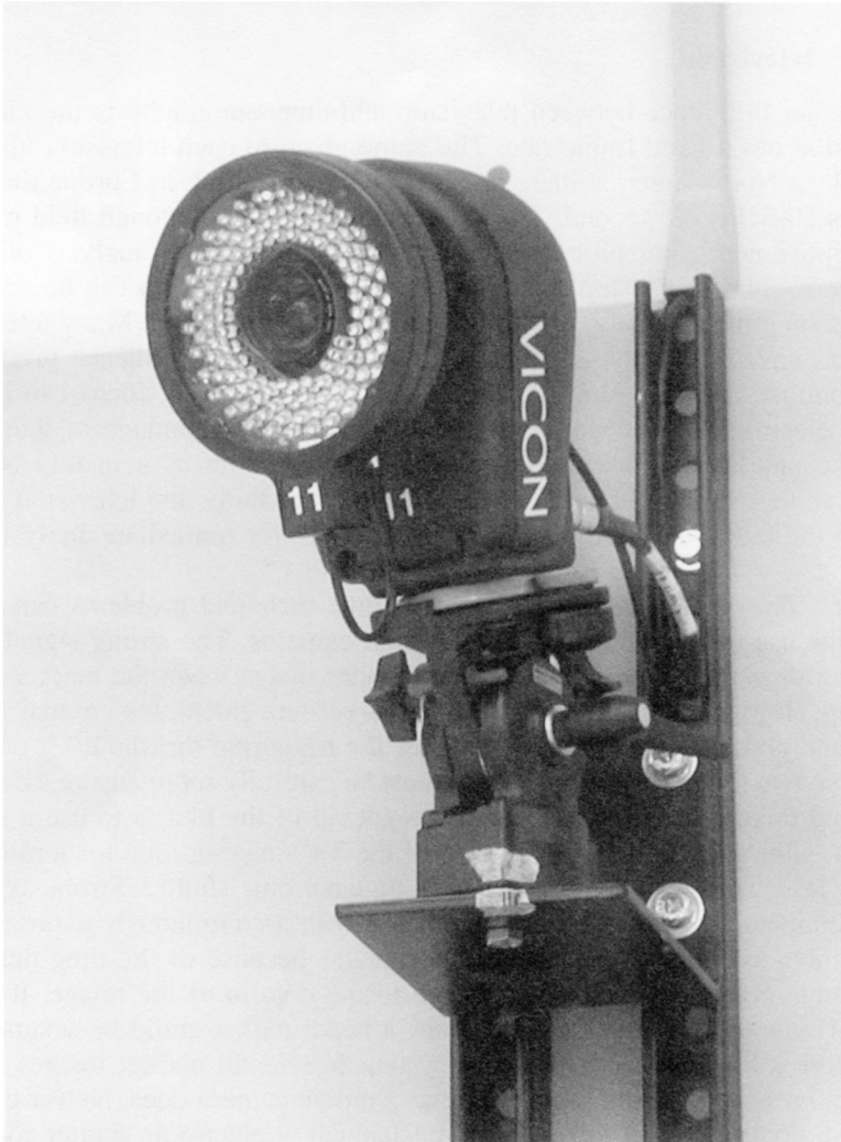
Figure 3.12 Typical infrared television camera mounted permanently in a clinical gait laboratory. The infrared lights form a “donut” shape around the lens and are pulsed for a short time each frame to freeze the image prior to scanning. (Courtesy of the Gait Analysis Laboratory, Connecticut Children’s Medical Center, Hartford, CT.)
