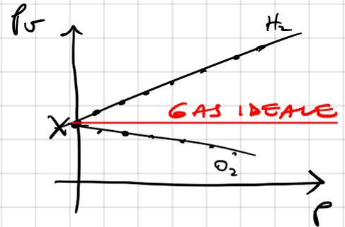
$$p_0 = \frac{pV}{w} = \lim_{p' \rightarrow 0} p' v' = X = \frac{X_{TP}}{273.16 \text{ K}} \quad T = RT$$
