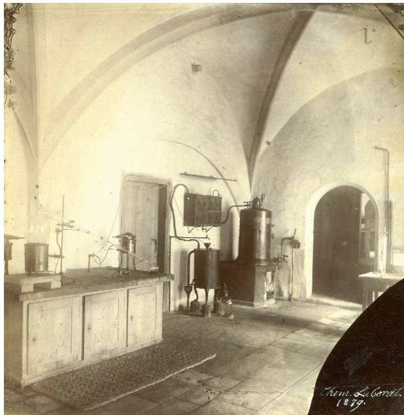
Fig. 4. The laboratory in the former kitchen of the castle in Tübingen as it was in 1879. It was in this room that Miescher had discovered DNA 10 years earlier. The equipment and fixtures available to Miescher at the time would have been very similar, with a large distillation apparatus in the far corner of the room to produce distilled water and several smaller utensils, such as glass alembics and a glass distillation column on the side board. Photography by Paul Sinner, Tübingen.
