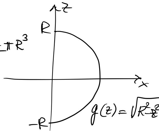
$$\begin{aligned} \text{vol } T &= \pi \int_a^b g(z)^2 dz = 2\pi \int_a^b \frac{g(z)^2}{2} dz = \\ &= 2\pi \int_a^b dz \int_0^{g(z)} x dx = \\ &= 2\pi \iint_E x dxdz. \end{aligned}$$
