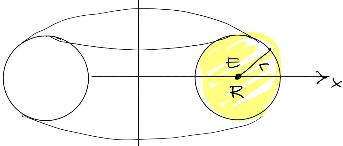
$$\text{vol } T = 2\pi \underbrace{\text{area } E}_{\pi r^2} \cdot \cancel{x_B} \stackrel{R}{=} 2\pi^2 r^2 R$$
