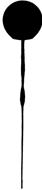
Figure 1.20 Photograph of a low-density, low-viscosity glucose fluid plume ascending in a high-density, high-viscosity glucose fluid (Olson and Singer, 1985).
