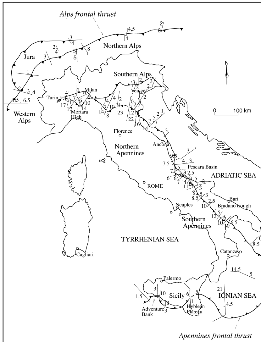
Fig. 2. Dip values of the regional monocline around the Alps and the Apennines. References in the text.
