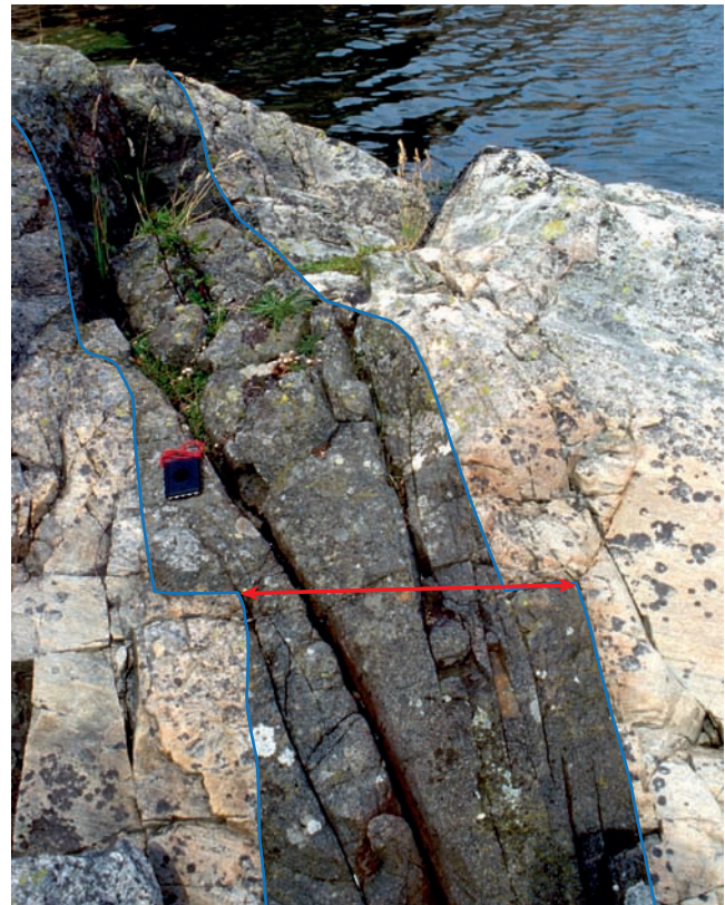
Figure 9.13 Left-stepping dike intrusion, well suited for stress determination. The corners were connected prior to the intrusion, and the extension direction, which can be assumed to be close to the minimum principal stress, is found by connecting the corners. Permian dike along the shoulder of the North Sea rift system.
