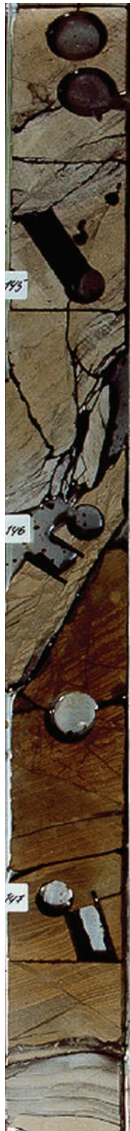
Figure 8.22 One-meter-long core section across a minor (6 m missing section) fault in the Gullfaks Field. Holes are from plugs sampled for permeability analysis. See also Figure 8.19.
