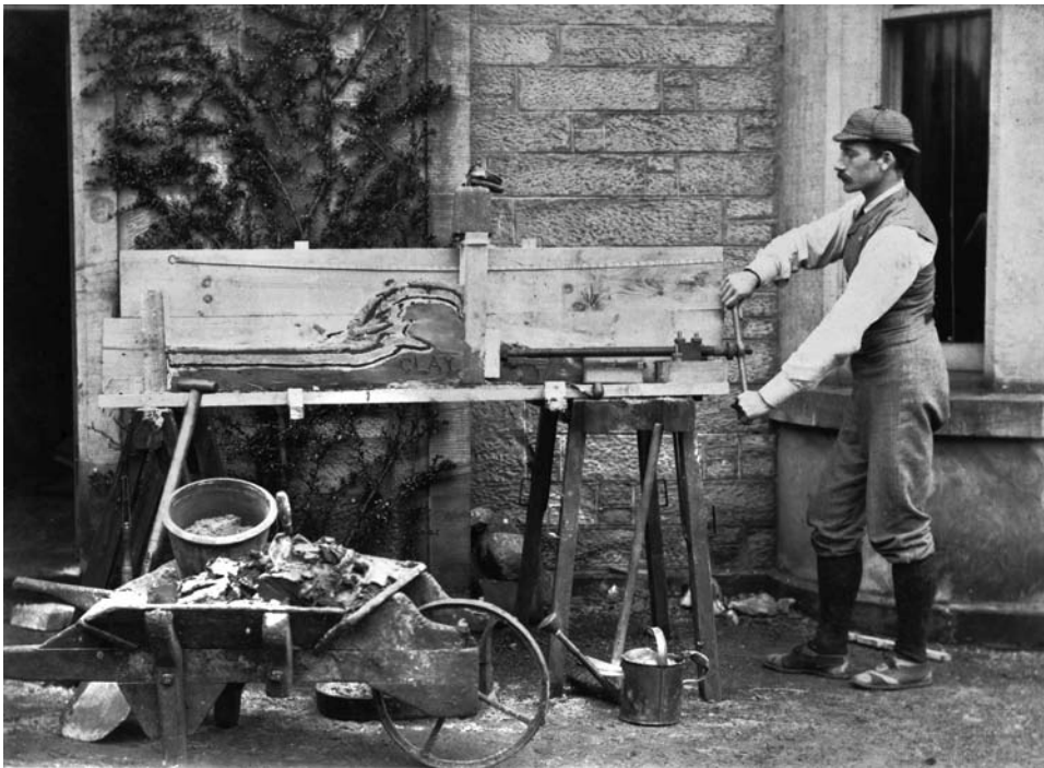
Figure 1.7 Experimental work in 1887, carried out by means of clay and a simple contractional device. This and similar models were made by H. M. Cadell to illustrate the structures of the northwest Scottish Highlands. With permission of the Geological Survey of Britain.
