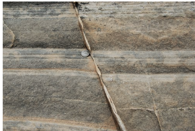
Figure 7.38 Cataclastic deformation band in porous Navajo Sandstone. The thickness of the band seems to vary with grain size, and the shear offset is less than 1 cm (the coin is 1.8 cm in diameter).
