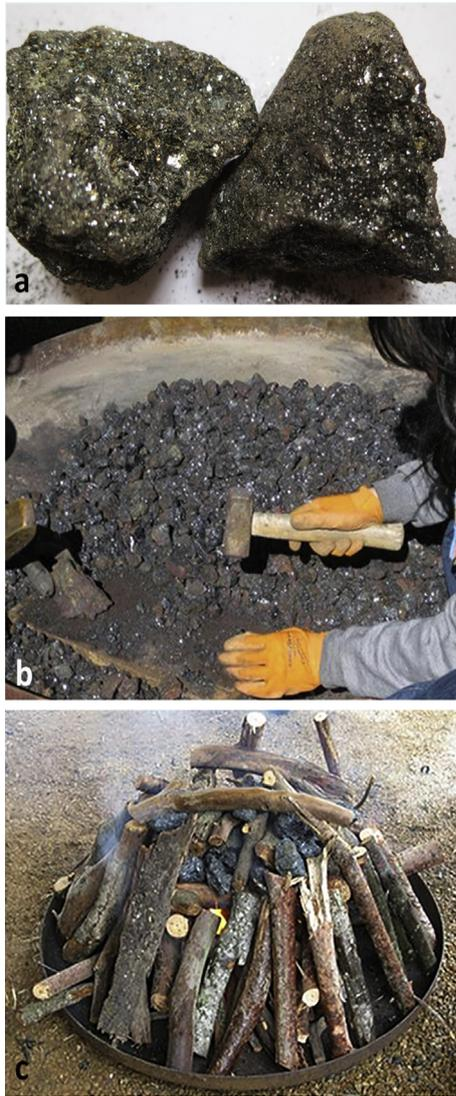
**Fig. 3.** (a) Run-of-mine iron ore (each ore fragment is approximately 10 cm large); (b) Ore crushing; (c) Roasting of iron ore to eliminate volatiles.
