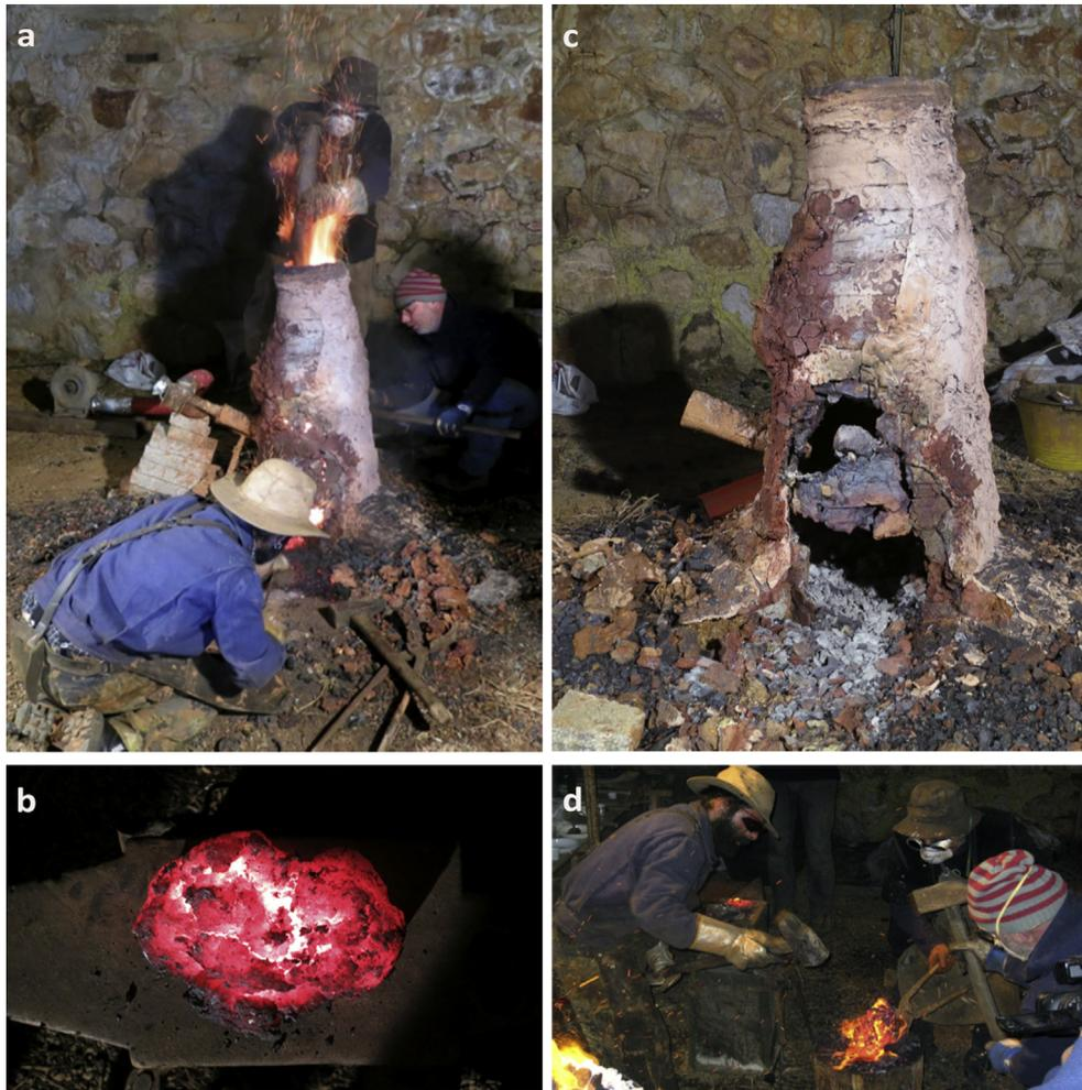
**Fig. 5.** (a) After breaking the basal plinth, the tap hole was opened and the front of the furnace partially wrecked to facilitate bloom removal; (b) Close-up view of one of the three pieces of iron bloom; (c) The furnace after smelting: note the intense thinning of the lower part due to reaction with the charge; (d) The bloom still hot was partially worked immediately after extraction from the furnace.
