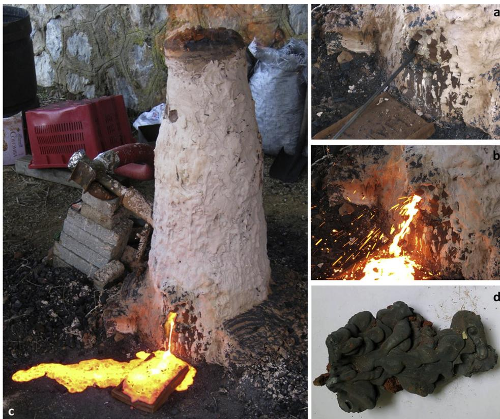
**Fig. 4.** (a) Breaking the front of the furnace for slag tapping out of it; (b) and (c) The first slag tapping; (d) a piece of slag tapped during the experiment.
