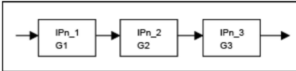
Figure 12. Cascaded RF functional blocks with known IPn.
