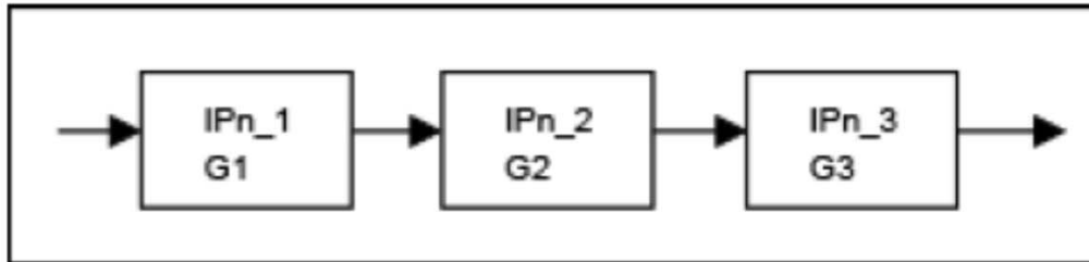
Figure 12. Cascaded RF functional blocks with known IP_n .
