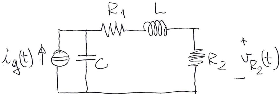
$$R_1 = 1\Omega; \quad R_2 = 1\Omega; \quad L = 1H; \quad C = 1F; \quad i_g(t) = \begin{cases} 1 & t < 0 \\ 0 & t \geq 0 \end{cases}$$
