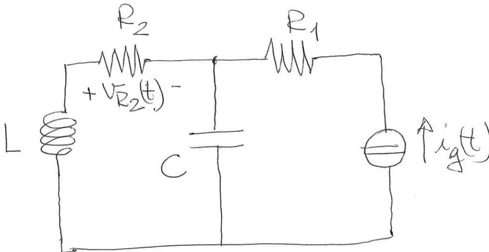
$$R_1 = 1\Omega; \quad R_2 = 1\Omega; \quad L = 1H; \quad C = 1F; \quad i_g(t) = \begin{cases} 1 & t < 0 \\ 0 & t \geq 0 \end{cases}$$
