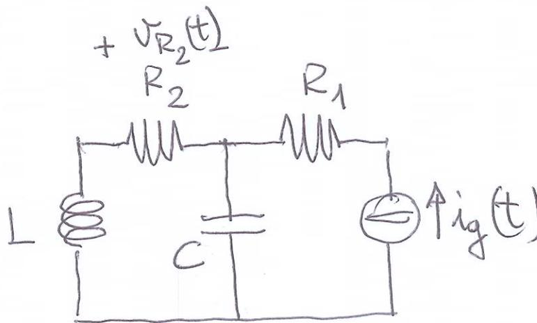
$$R_1 = 1\Omega; \quad R_2 = 1\Omega; \quad L = 1H; \quad C = 1F; \quad i_g(t) = \begin{cases} 1 & t < 0 \\ 0 & t \geq 0 \end{cases}$$
