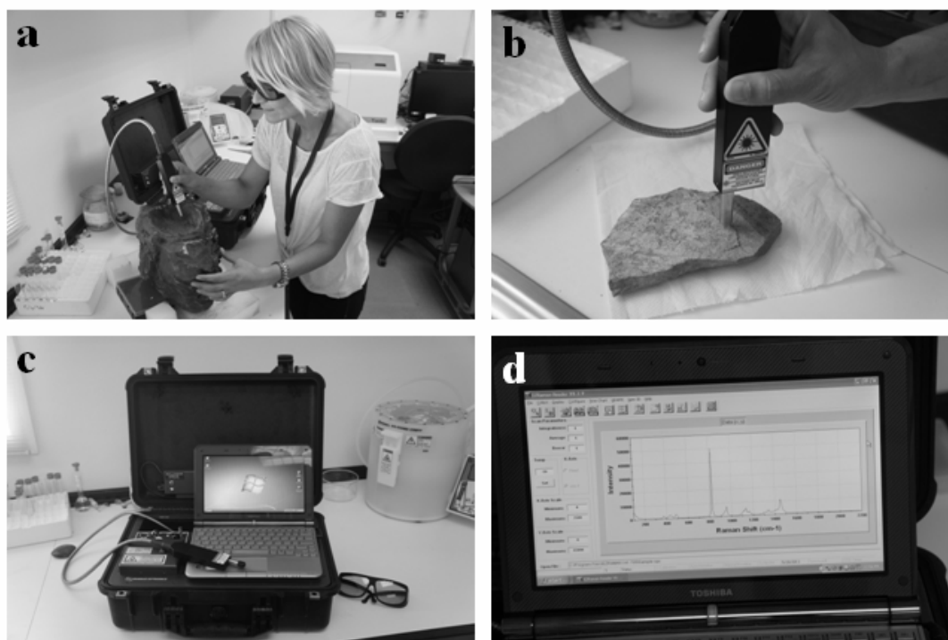
Figure 1. Raman spectroscopic analysis performed by means of a portable instrument of (a) a prehistoric stone lamp and (b) a lithic instrument with traces of pigments. c. Portable Raman spectrometer equipped with an optical fiber and a head probe. d. Raman spectrum performed with a portable spectrometer.
