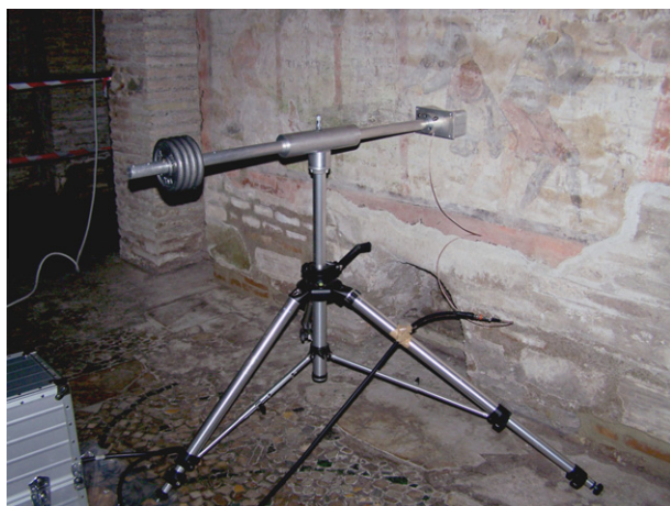
Fig. 7. Unilateral NMR instrument measuring the moisture content in the St. Clement at mass and the legend of Sisinnius wall painting, St. Clement Basilica, Rome.
