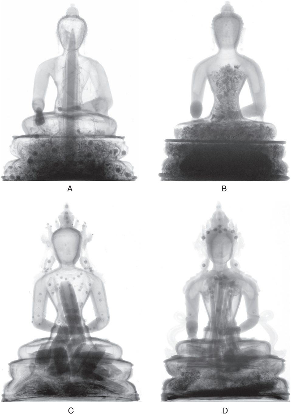
Figure 5 Frontal transmission neutron radiography images of the four Buddha objects (see Table 1); the description as sample A–D is used consistently.
