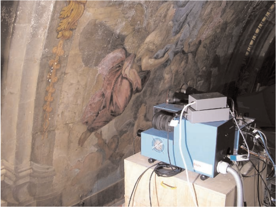
FIGURE 5.33 Laseract Multitask system for onfield investigation of wall painting.
