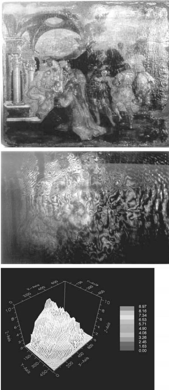
FIGURE 5.22 (See color insert.) The interferogram revealed highly irregular fringe distribution with extended superficial detachments and defect propagation affecting the whole front surface to react as loosely attached to frame membrane.
