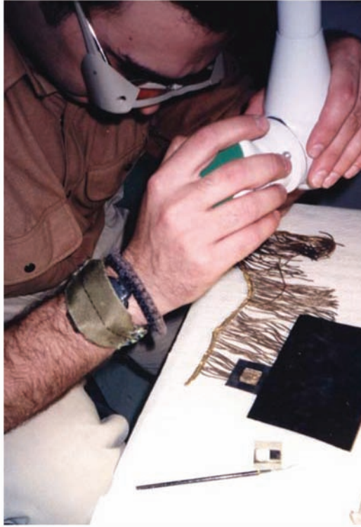
FIGURE 9.6 Laser cleaning of fringes with silk core and tarnished gilt silver threads.
