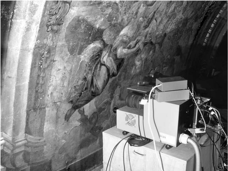
FIGURE 5.33 (See color insert.) Laseract Multitask system for onfield investigation of wall painting.
