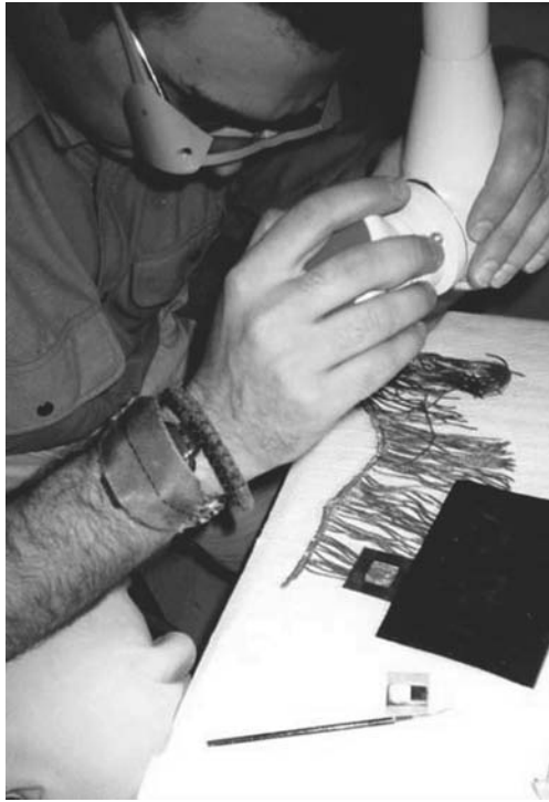
FIGURE 9.6 (See color insert.) Laser cleaning of fringes with silk core and tarnished gilt silver threads.
