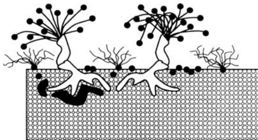
FIGURE 9.2 Molds may grow into the paper substrate, produce stains by metabolizing trace metals in the paper, produce fruiting bodies that can imbed themselves in the paper and develop into new mold colonies, or initiate cellulolytic processes that destroy the paper matrix.
