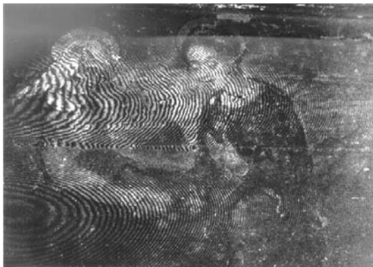
FIGURE 5.17 Painting exhibiting two whole-body fringe systems generated by panel separation along a central x -axis. The difference in the density of fringes visualizes the differential response of the upper in comparison to the lower part due to missing canvas at the lower region.
