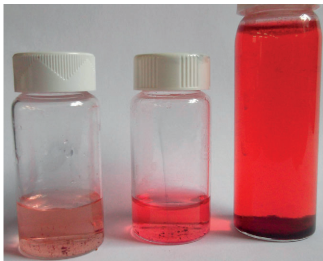
Figure 7. Saturated solutions of: pseudopurpurin in water (left); pseudopurpurin in 5% alum solution (centre); and R. tinctorum root (previously soaked in water and dried) in 5% alum solution (right)
