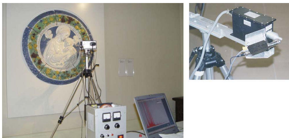
Fig. 1. The portable EDXRF spectrometer used in this work.
