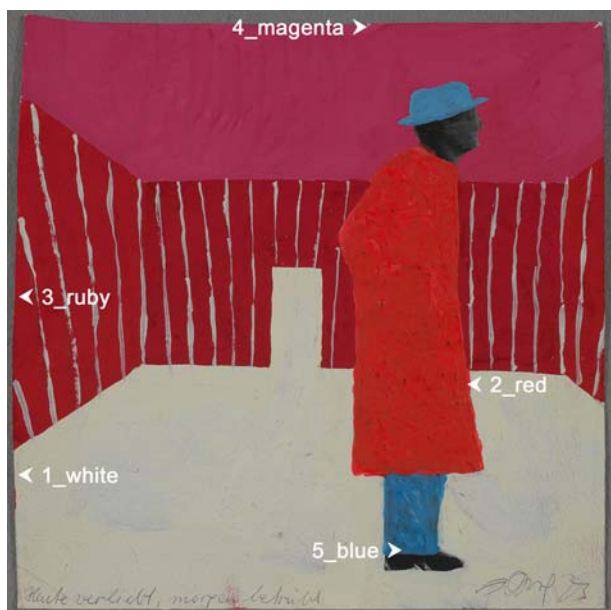
Figure 14: Painting on paper (Inv. No. DN 2181) with the title "Heute verliebt, morgen betrübt" by the contemporary artist Franz West including the points/areas used for r-FTIR and \mu -FTIR.
