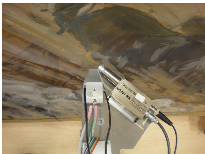
Fig. 2. The portable EDXRF spectrometer during analysis of the Sorolla's gouache sketches.
