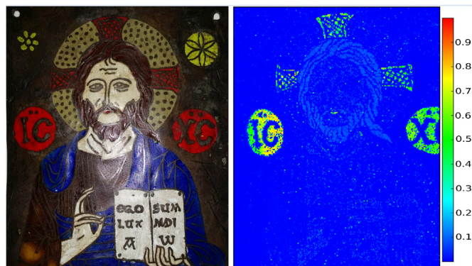
Fig. 4. Elemental map associated to NNMA spectrum of Fig. 3.
