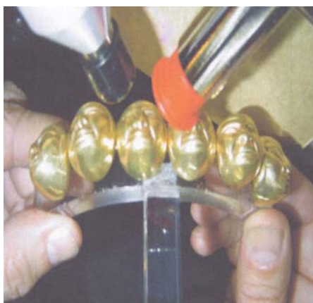
Fig. 11 Complex of six small heads of Chavin culture (Museo Poli, Lima), possibly on tumbaga. Following was determined: Cu(K_{\alpha}/K_{\beta}) = 4.5 \pm 0.2 , corresponding to an equivalent gold thickness of 2 \mu\text{m} . The composition of the internal copper was determined to be: Cu = 98.5\% , Zn = 1.5\% , Fe = \text{traces} . X-Ray tube (top left) and Si-drift X-ray detector (top right) are also visible.
