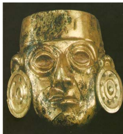
Fig. 17 Mask made of gilded copper from the tomb n. 3 of “tumbas reales de Sipán” Areas relatively free from Cu-compounds have been analyzed. A gilding thickness of \sim 0.6 \mu\text{m} was determined.
