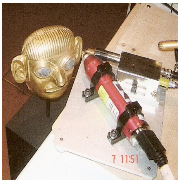
Fig. 2 Experimental set-up, showing, on the left, the Eclipse II X-ray tube (collimated with a brass cylinder), with Ag-anode and working at 30 kV, 100 \mu A maximum voltage and current, and the Si-PIN detector (also collimated with a brass cylinder), during measurements on the golden mask, in the Museum “Tumbas Reales de Sipán”. A typical measurement takes 50-200 s, depending on the geometry and object composition.
