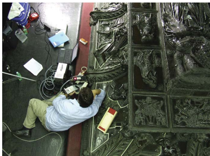
Fig. 2. The portable EDXRF equipment in operation during the measurement on the monument in restoration; detail of the probe and operator at work.
