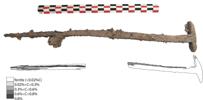
Fig. 2. Sample iso37096 from Castel-Minier archaeological site (Ariège, France). Schematic drawing of the microscopic metallographic observation on the cross-section after Nital etching.
