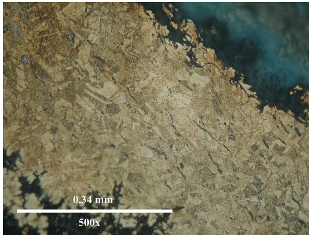
Fig. 5 Photomicrograph of the etched section of Gomolava ring (sample No. 212), with significantly reduced grain structure, deformation marks and elongated sulphur-rich inclusions, all of which suggests several cycles of annealing (Radivojević et al. 2013, 1039, Fig. 6)
