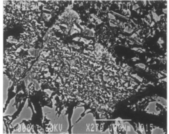
Fig. 3. Dublin. Contact between gypsum patina and granite showing a feldspar mineral totally replaced by gypsum. Note how the original outline of the silicate mineral can still be seen.
