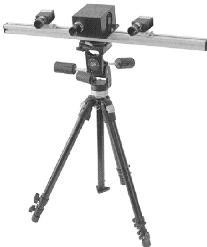
Fig. 1. The scanning system: a solid bar mounted on a tripod holding a projector positioned between two cameras.
