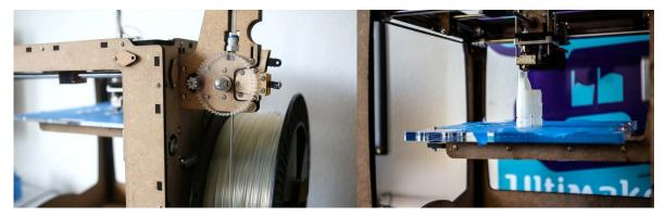
Fig.1: View of the Ultimaker®: a 3D printer used for the manufacturing of the PLECO. ©FabLab-Neuch
