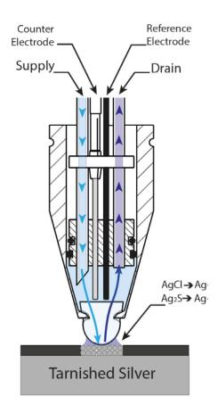
**Fig. 5:** Sectional view of the PLECO electrolytic cells. ©HE-Arc CR
