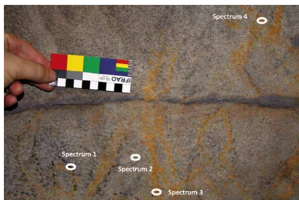
Figure 5 Detail of the rock art panel. The white ovoids indicate the location and approximate size of the PXRf instrument aperture. In Situ Loci 3 (i.e. Spectrum 3) is the location of previous pigment harvesting (photograph by Jillian Huntley).
