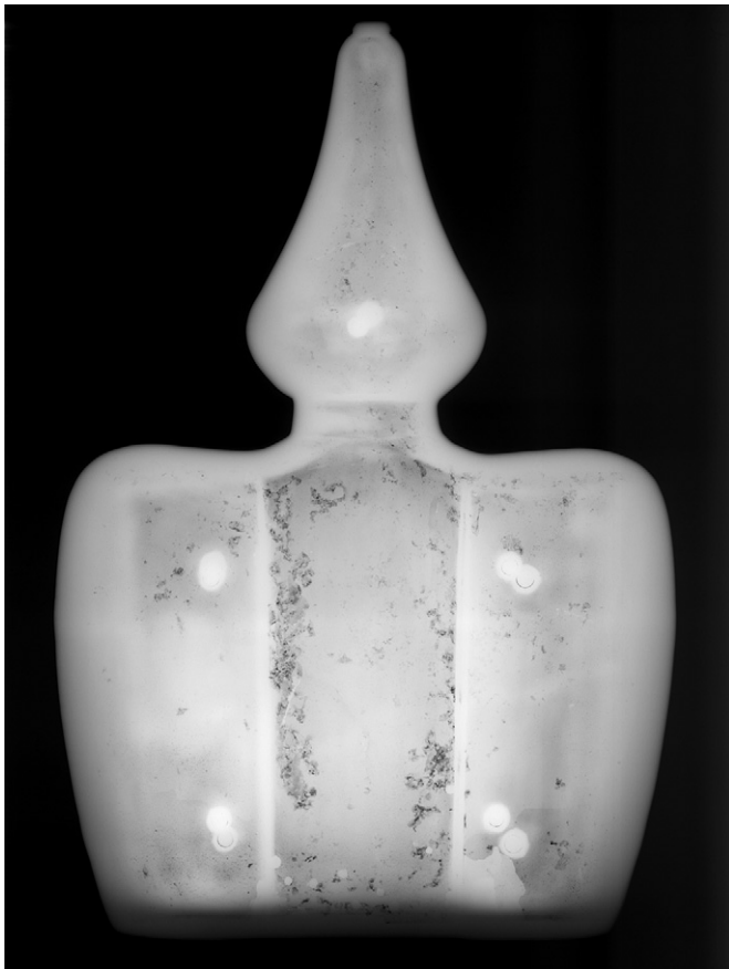
Fig. 12. X-ray image of a phytomorphic vessel showing porosity areas (darker) and the symmetrical position of the perfectly circular holes (brighter) of the inner core sustaining pegs. Museo de América, Madrid (photo: Archivo Gabaldón-Antelo, IPCE).
