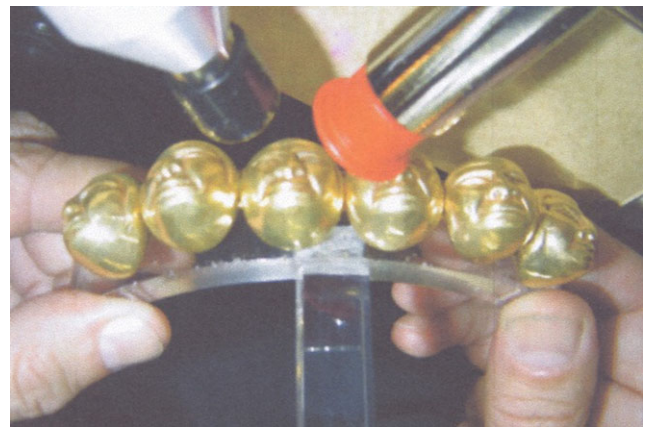
Fig. 8 Complex of six small heads of Chavin culture (Museo Poli, Lima), possibly on tumbaga, or, less probably, on gilded copper. X-ray tube (top left) and Si-drift X-ray detector (top right) are also visible
