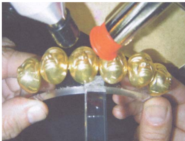
Fig. 11 Complex of six small heads of Chavin culture (Museo Poli, Lima), possibly on tumbaga. Following was determined: Cu(K_{\alpha}/K_{\beta}) = 4.5 \pm 0.2 , corresponding to an equivalent gold thickness of 2 \mu m . The composition of the internal copper was determined to be: Cu = 98.5\% , Zn = 1.5\% , Fe = \text{traces} . X-Ray tube (top left) and Si-drift X-ray detector (top right) are also visible.
