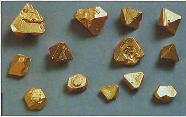
Figure 1a Faked octahedral gold crystals in the 1 to 30 gram range purported to come from the Santa Elena gold mine (Venezuela). Photo by P. Vollenweider.
