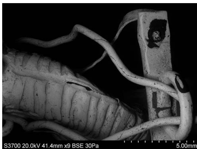
FIGURE 12. Backscattered electron image of the head of a horse with part of the yoke and a soldered terret through which two twisted wires – the reins – pass
