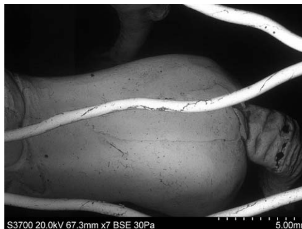
FIGURE 15. Backscattered electron image of the back of one of the horses where it has been mended, probably in antiquity, with an added piece of gold soldered onto the original body
