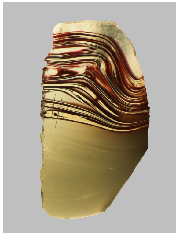
Fig. 21. Cross-section of an original, rounded (not grozed) edge (right hand side of image) of red type A from Chapter House (w1, window tracery), Canterbury cathedral, probably 14th century. Lines from laser scan may be observed centre left. (For interpretation of the references to colour in this figure legend, the reader is referred to the web version of this article.)
