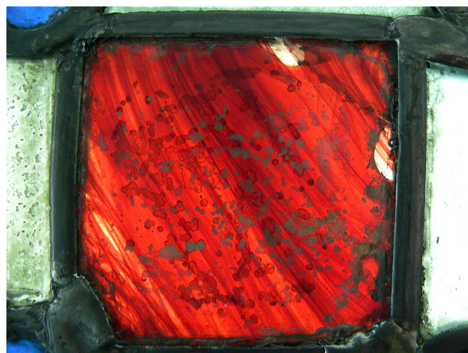
Fig. 14. In situ type A with ‘wavy’ pattern due to the uneven distribution of red striae. Canterbury cathedral, 12th century. (For interpretation of the references to colour in this figure legend, the reader is referred to the web version of this article.)
