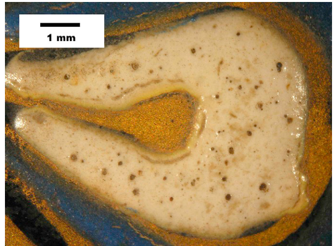
Fig. 12. White cold ground enamel of MAO 490/41. Irregular aspect with bubbles and cracks probably due to a very short firing.
