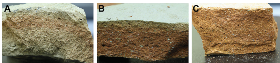
Fig. 3. Macro photograph of some representative samples showing the colour variation along the section: A) Gela 103 sample, with a thick whitened layer and a light pink core; B) Gela 76 sample, with a thin whitened superficial layer and a red core; C) Gela 40 sample, without whitening.
