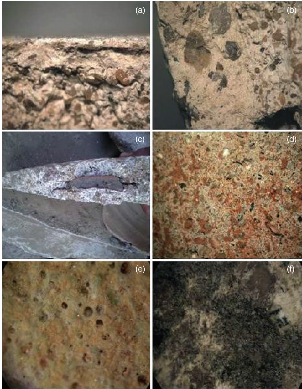
Figure 2 Stereomicroscopic images of the studied plaster layers. (a) A stratigraphical section in the plaster layers. (b) A close-up of the coarse plaster layer. (c) A cross-section in a plaster layer shows the pottery sherd brick embedded in the plaster layers. (d) A superficial image of the red pictorial layer. (e) A detail of the yellow pictorial layer. (f) A detail of the black pictorial layer.
