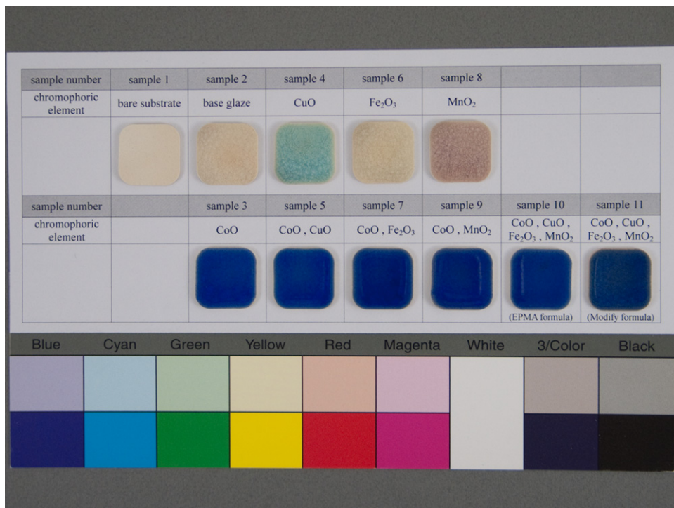
Figure 11 A colour comparison of bare substrate, the base glaze and glazing samples doped with individual and mixed chromophoric elements.
