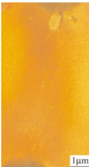
Figure 7. LOM micrograph showing the joint analyzed with LISPIX. Etched with Aqua Regia, unpolarized light.
