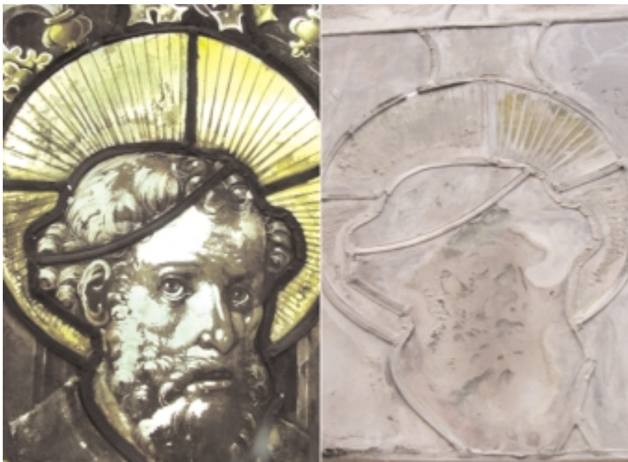
Figure 1. Detail of the panel 6 window sIII, Cathedral of Avila. Photographs were taken with transmitted and reflected light. A dense weathering crust is reducing the transparency of most glasses.
