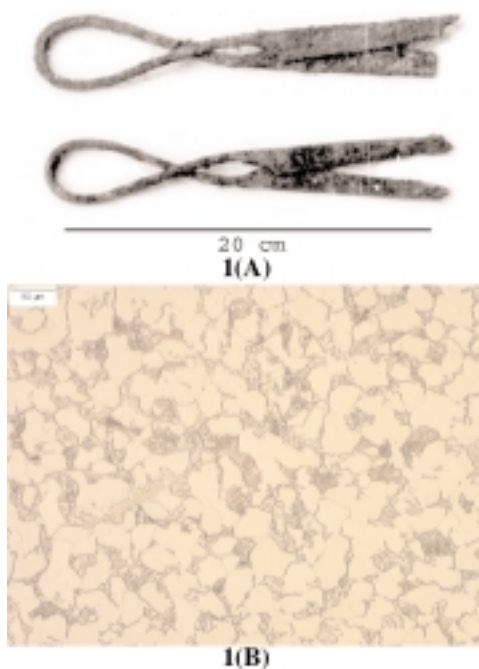
Figure 1. A) Sample 706 was taken from one of the two shears above, both excavated together [2]. B) LOM micrograph of the microstructure from sample 706. Note the absence of slag and the large pearlite lamellar spacing indicative of a decarburized cast iron. Etched 4% Picral, unpolarized light.
