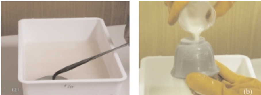
Figure 1. Examples of glaze application techniques a) full dipping and b) pouring.
