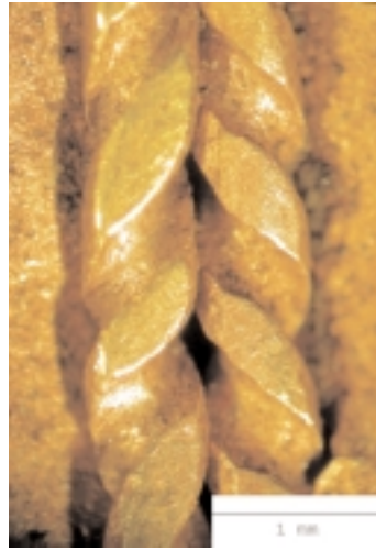
Figure 3. Photograph, in unpolarized light, of the simulated wire braiding on the filigree. The edges display that this is twisted flat strip.
