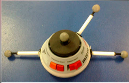
Figure 2: Dynamometer with the four markers.
