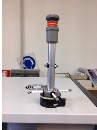
Fig. 10: Load cell equipped with markers
