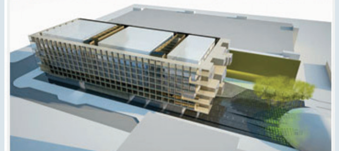
Cubiform offices on the perimeter wrap around white laboratory volumes separated by the atriums.
