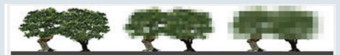
The architects pixelated an image of two trees to morph the organic form into Cartesian geometry for the building's design.
