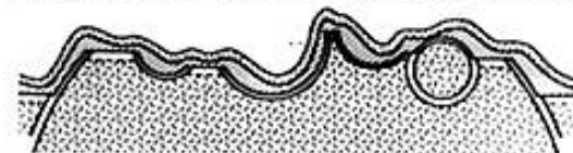
Replication of Fractured Surface
