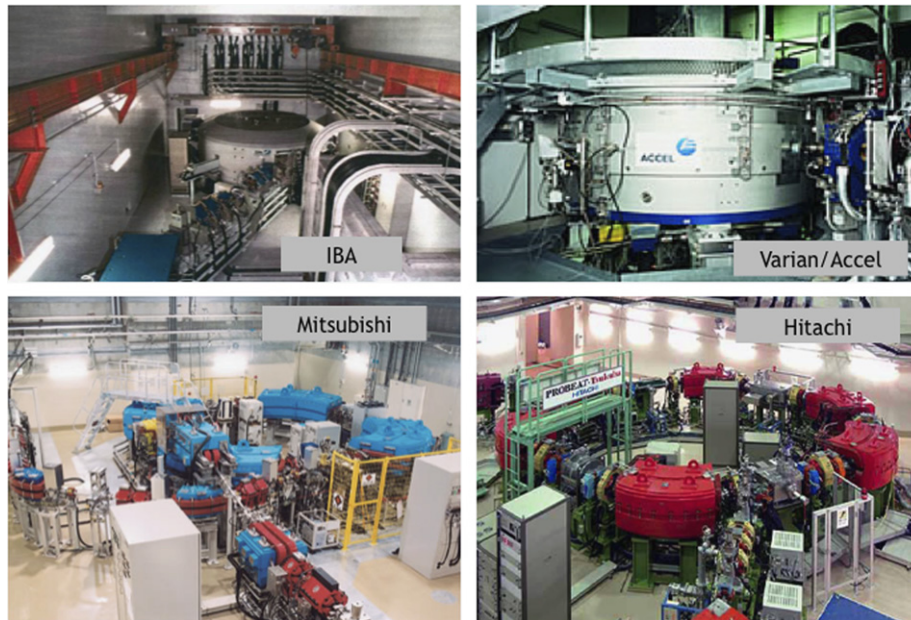
Fig. 3. Commercial accelerators for proton therapy: cyclotrons (by IBA and Varian/Accel) and synchrotrons (by Mitsubishi and Hitachi).
