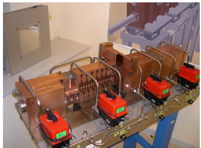
Fig. 7. Picture of the four ‘tanks’ of the LIBO prototype. Each tank is made of a number of basic units machined with high accuracy in copper and called ‘half-cell-plates’. The cut-out shows the structure of the accelerating and coupling cells.
