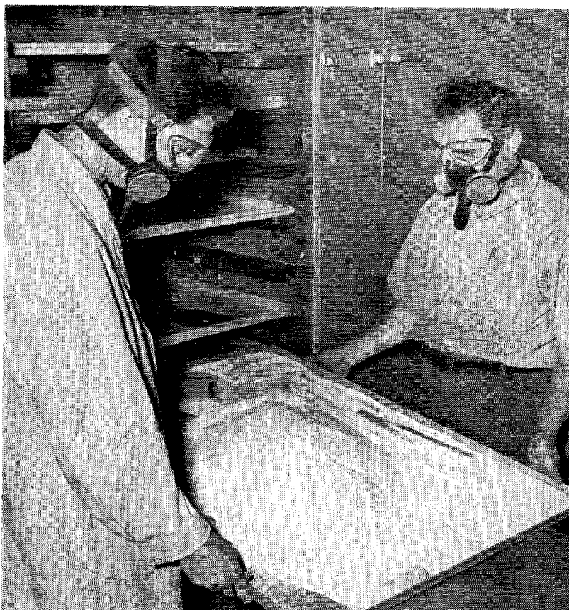
Figure 5. Operators Removing Aralen from Drying Oven
