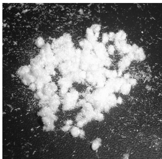
Figure 1. Crystals of quinine tartrate obtained directly from quinotoxine according to the Rabe–Kindler protocol [2] without the use of any modern isolation, chromatographic, or analytical techniques.
